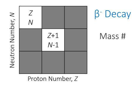
$$^{234}_{90}\text{Th} \rightarrow ^{234}_{91}\text{Pa} + ^{0}_{-1}\text{e} + \bar{v}_{e}$$
