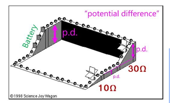
The voltage used by the resistors equals the voltage supplied by the battery Each resistor has a "voltage drop"
