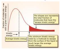
When these faster molecules are lost, the average KE of the liquid decreases, resulting in evaporative cooling
