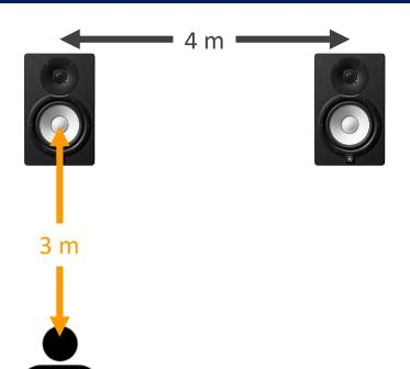
If these speakers are playing a note with a frequency of 680 Hz, is this person standing at a maximum or minimum spot? Assume a speed of sound of 340 m s<sup>-2</sup>
