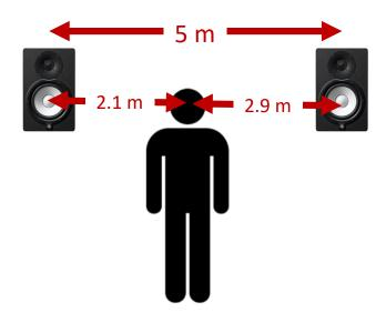
Two speakers are separated by a distance of 5 meters, if they emit a coherent sound signal of 850 Hz. If the speed of sound is 340 m s<sup>-1</sup>, is this person in a maximum or minimum location?
